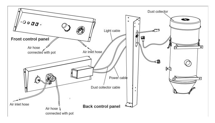
Steps 11: Connect electrical parts and quick air couplings. Please note wrap the sealing tape when assemble connector and quick air coupling to avoid air leaking.
